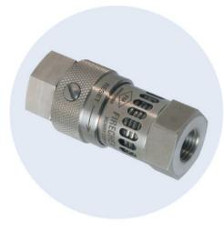
When FireChek senses excessive heat from a nearby fire, it immediately vents the pneumatic actuator and closes the actuator air supply line. FireChek triggers quickly, securing pneumatically operated process line valves. Because FireChek responds to heat, not flame, it offers dramatically improved protection compared with conventional plastic tubing burn-through. It shuts off the air supply line to prevent plant air from feeding oxygen to a fire.
